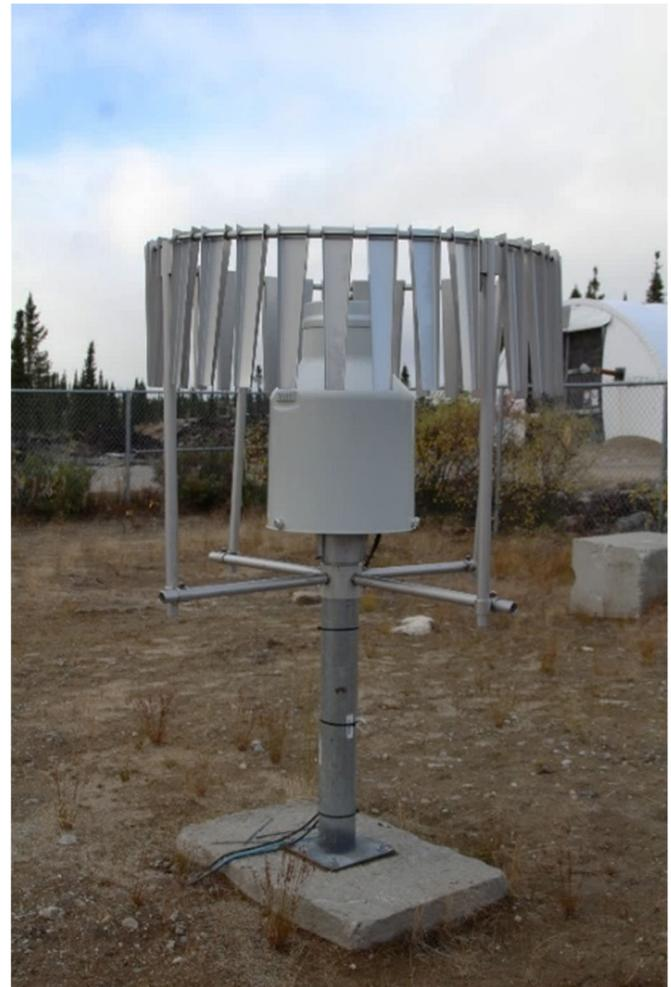
**Photo 3.2 Precipitation gauge near weather station**
