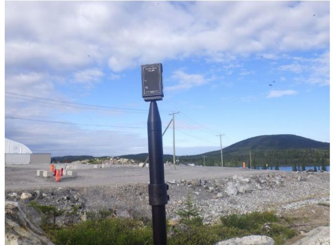
**Photo 3.12 Calibration of sonometer used in acoustic monitoring surveys**
