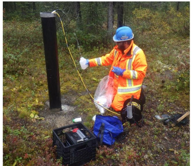
Photo 3.56 Groundwater sampling at the TLS (September 2019)
